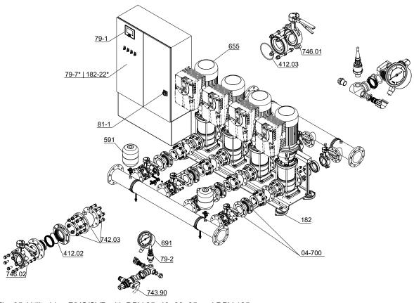
Fig. 25: Utility Line F/VC/SVP with DPV 25, 40, 60, 85 and DPV 125
