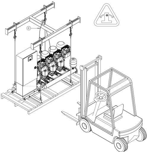
Fig. 3: Lifting the pressure booster system and control cabinet together on one baseplate 1. Use anti-tilting device C.
