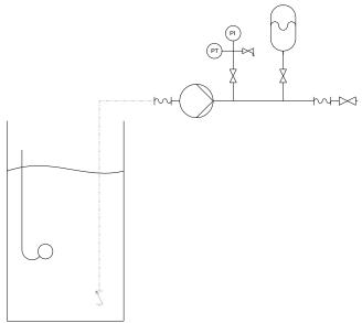
Fig. 13: L = Pressure booster system with break tank arranged at a lower level, suction lift operation
