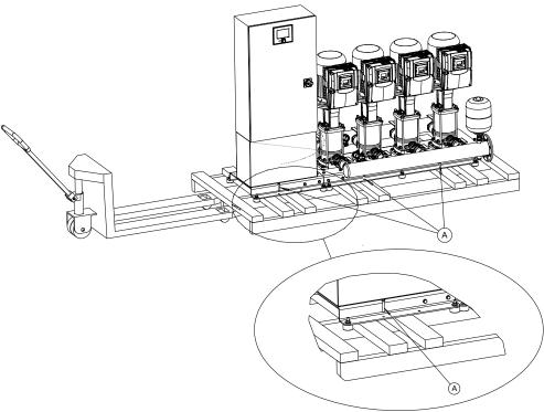
Fig. 1: Lifting the pressure booster system off the pallet
