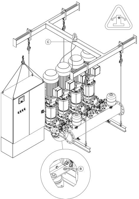
Fig. 2: Lifting the pressure booster system and control cabinet separately
