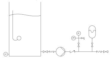
Fig. 11: F = Pressure booster system with break tank arranged on same level as pump, suction head operation
