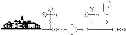
*Fig.* 9: M = Inlet side of pressure booster system connected to the municipal water supply, suction head operation
