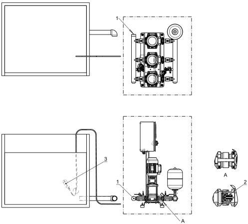
Fig. 12: Scope of supply, version F
